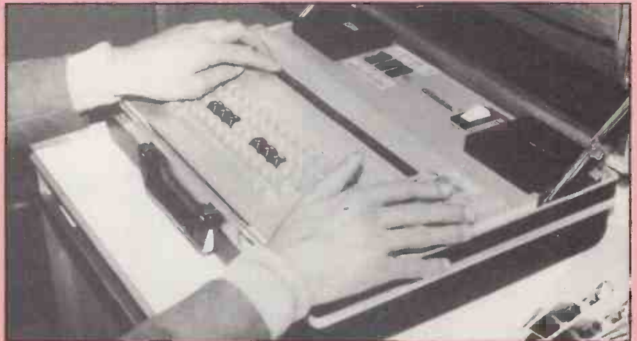
Linked to the Brailink terminal, Prestel can display information in Braille.
