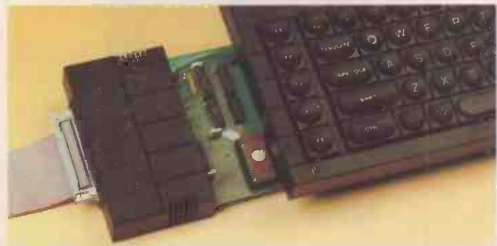
A Centronics interface slips discreetly into place.
